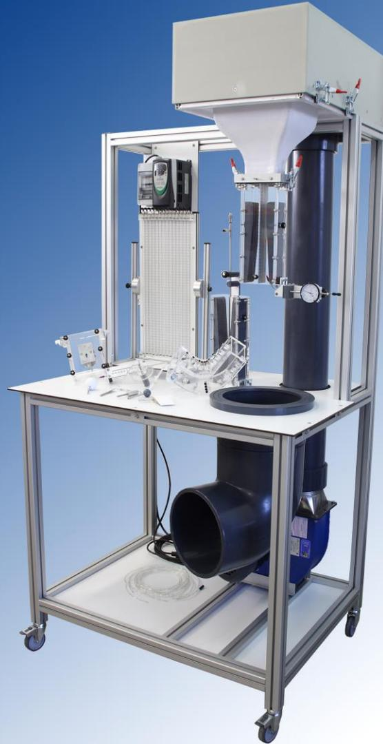
The aerodynamics bench is designed to perform a variety of experiences in the field of fluid mechanics, using a controlled airstream for it.
