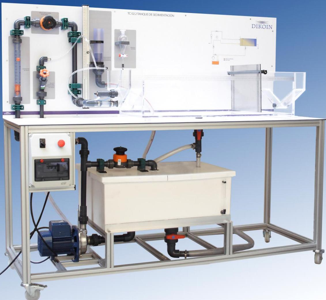
With this equipment is intended to study and visualize in a continuous regime, the natural phenomenon called sedimentation, whereby particles that are denser than the fluid that contains them and in which they are dispersed, fall by gravity depositing in the bottom of the container.
