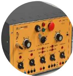
A three-phase power supply with fixed and variable outputs in AC and DC that provide the electrical power to the test bench and machines under study. The power supply includes all the protections needed to create a safe work environment for the student.
