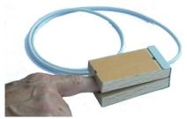
At every heartbeat the arterial blood pressure raises (systolic period) and the dimension of the tips of the fingers slightly increases, while the higher oxygenation causes the decrease of the optical density of the skin tissue.
