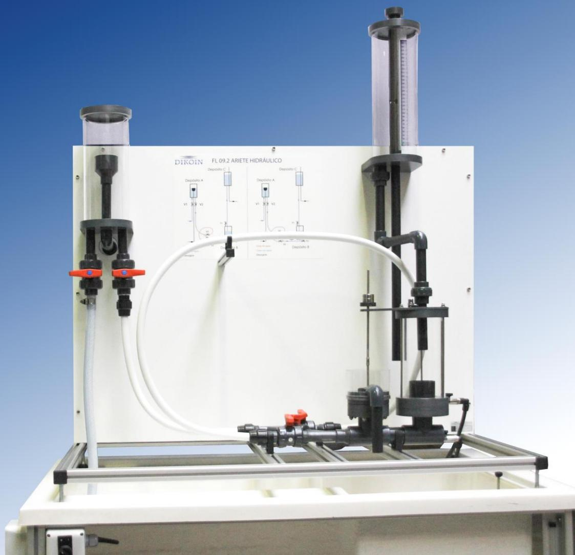
The FL09.2 is a equipment that aims to demonstrate and study the phenomenon known as water hammer, this phenomenon is the one that occurs due to the rapid closure of the passage of water through a pipe. The design of the equipment is made with special emphasis on the didactic field, so it is supplied with variable elements, to achieve a greater number of tests for a better understanding of the student.
