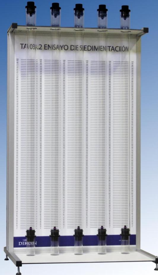
The objective of this equipment is to study and visualize the natural phenomenon called sedimentation, whereby the particles denser than the fluid that contains them and in which they are dispersed, fall by gravity depositing in the bottom.
