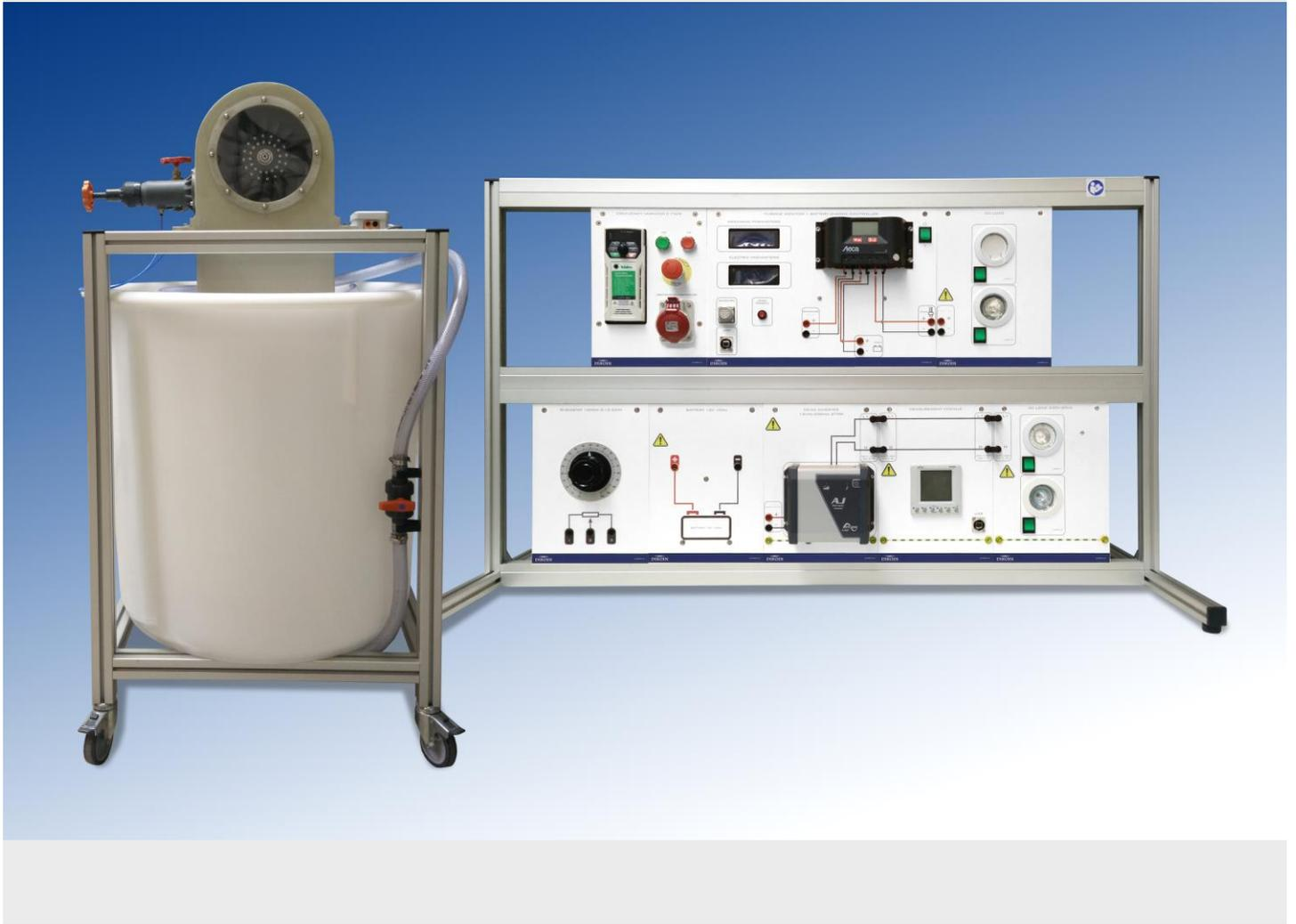
Trainer EN 05.1 has been designed as a small-scale hydropower plant and it is equipped with a Pelton turbine that provides full operation along with all the other accessories that complete a standard installation.
