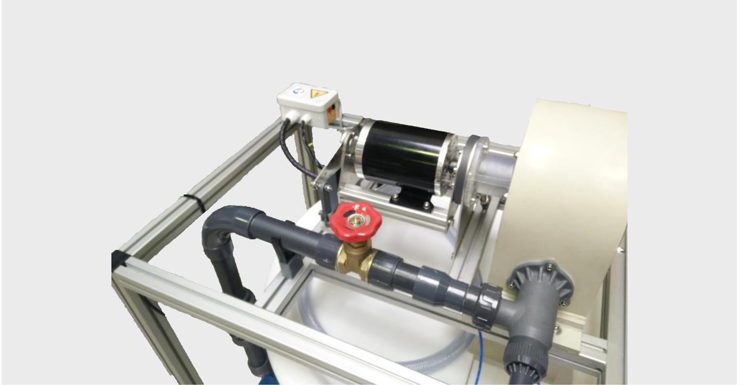
The construction shape of the equipment allows to visualize the entire process of transformation of hydraulic / mechanical / electrical energy.
