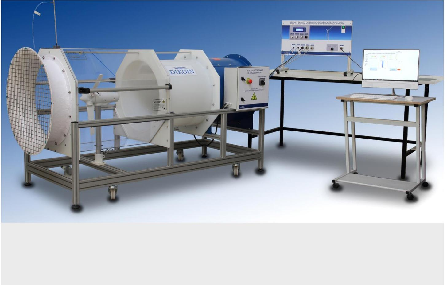
The Windmill Test-bench (EN 04.1), is a wind tunnel of 2 meters length designed to work with windmills of less or equal to 630mm diameter. The equipment has a 612 mm windmill included, which has a torque and rotation speed measurement system.
