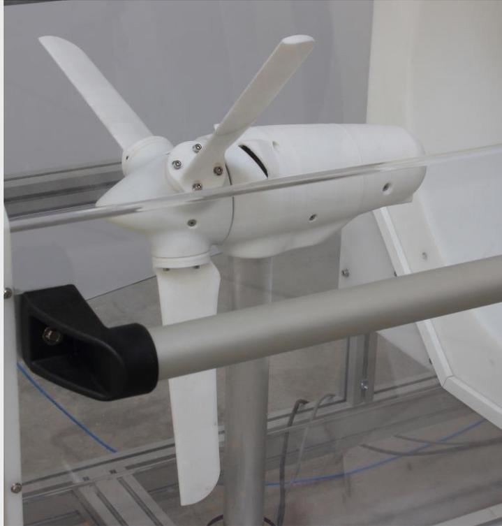
The turbine is fully developed and manufactured by DIKOIN, and has electronic speed and torque measurement systems. It also has an electronic pitch regulation system.
