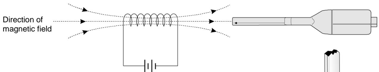
The Sensor can be positioned in either a horizontal or vertical position when using the **Radial** range to detect the field from a magnet.
