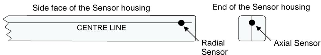
The two Hall Effect devices are located immediately behind the moulded circles on the sensor housing. The axial device is 2.35 mm behind the circle on the end face, and the radial device is 2.85 mm behind the circle on the side face. Each device is approximately the same size as the circle.
