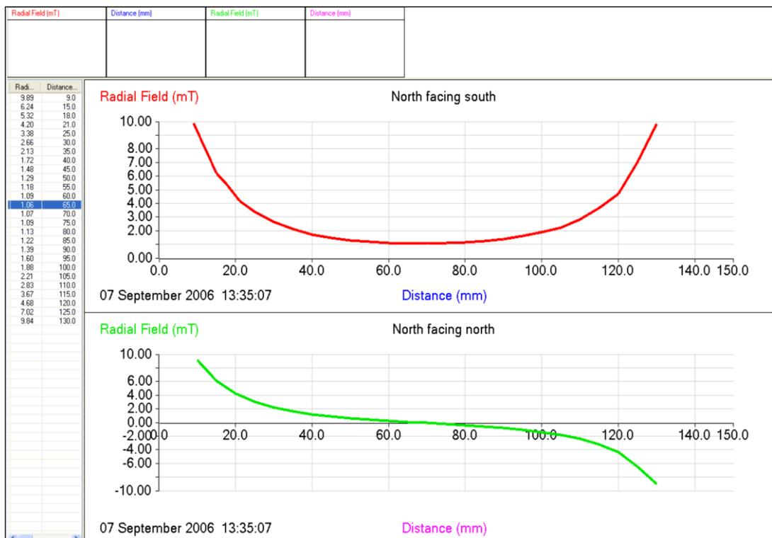
**The variation of magnetic field along the axis of a coil**
