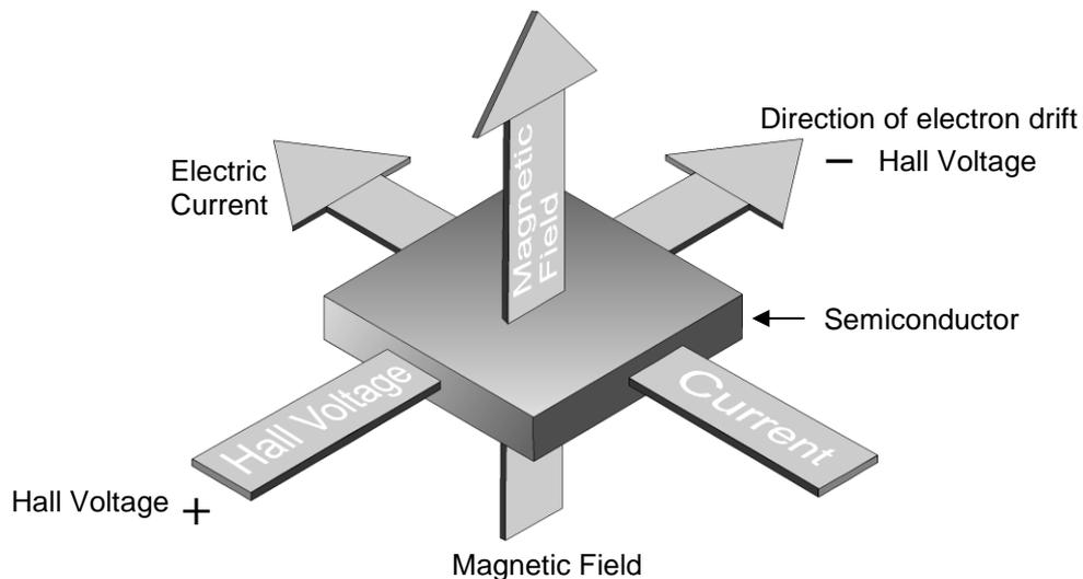
There are two Hall Effect devices in the Sensor, placed at right angles to each other. This enables fields along the axis of the Magnetic Field sensor (the axial field) or at right angles to it (the radial field) to be measured.
