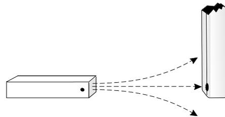
The Sensor can be positioned end-facing when the **Axial** range is used to detect the field from a magnet.
