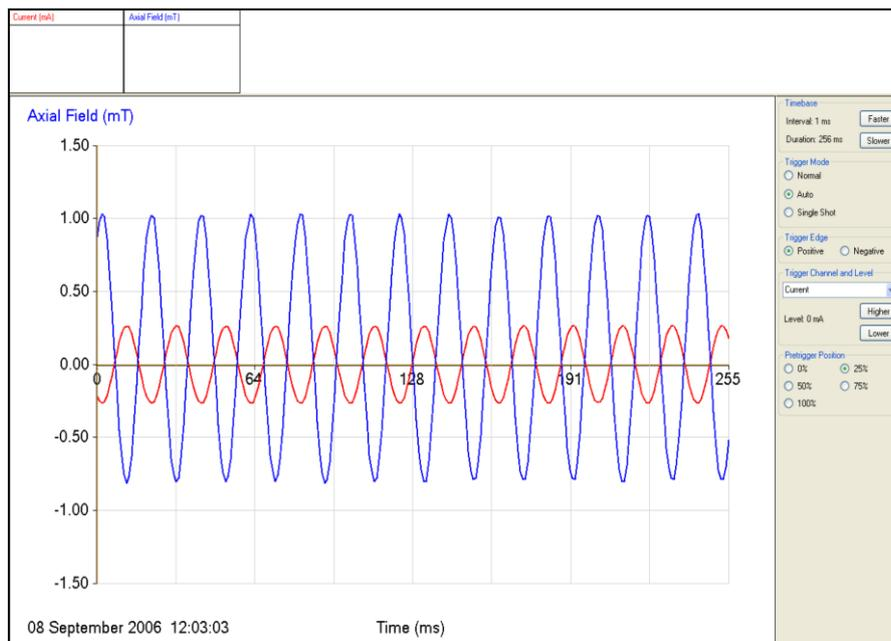
These results were obtained using a 350-turn coil and the 10 mT sensor
