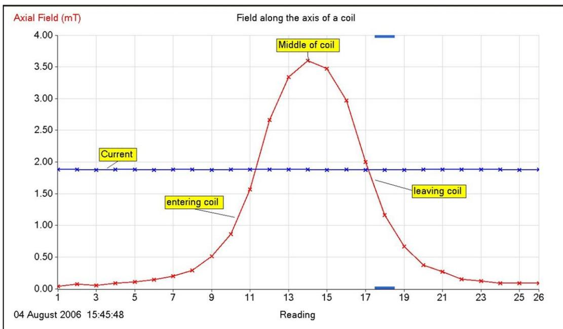
Result using a 200 turn 'home made' coil and 4.5 V d.c. from a power supply. Axis limits reduced to display from 0 to 4 mT.
