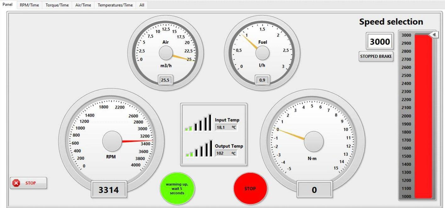
The equipment includes a PC with the equipment management software. In the same the parameters of all control points of the equipment are shown, and the data collection is allowed in automatic or manual mode.
