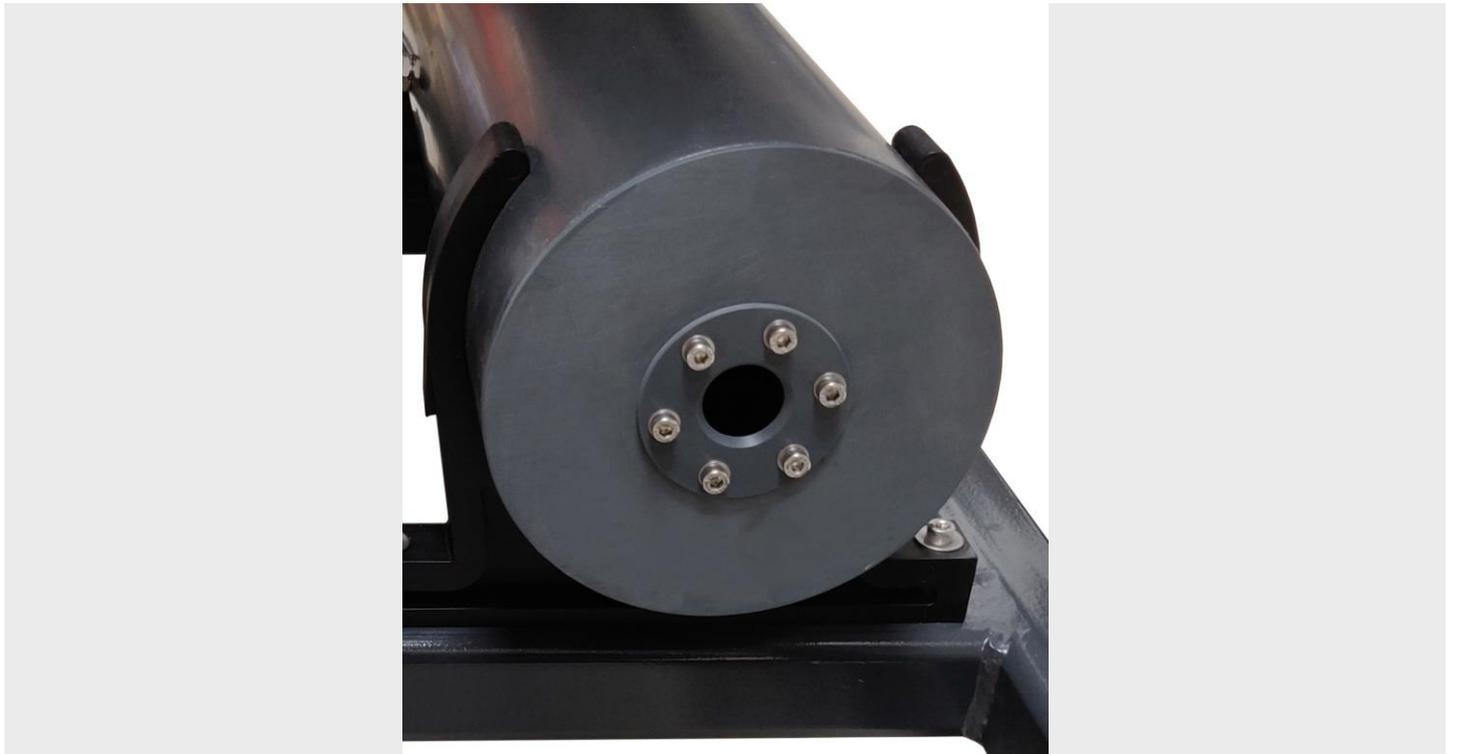
The system has a device for measuring the volume of air sucked by the engine, so that calculations can be made corresponding to the air-fuel ratio, etc.
