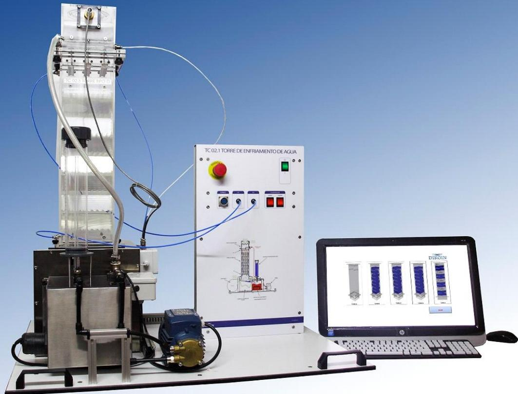
The TC 02.1 unit operates a standard cooling method, used in the industrial sector. This method involves cooling hot water to environment temperature.
